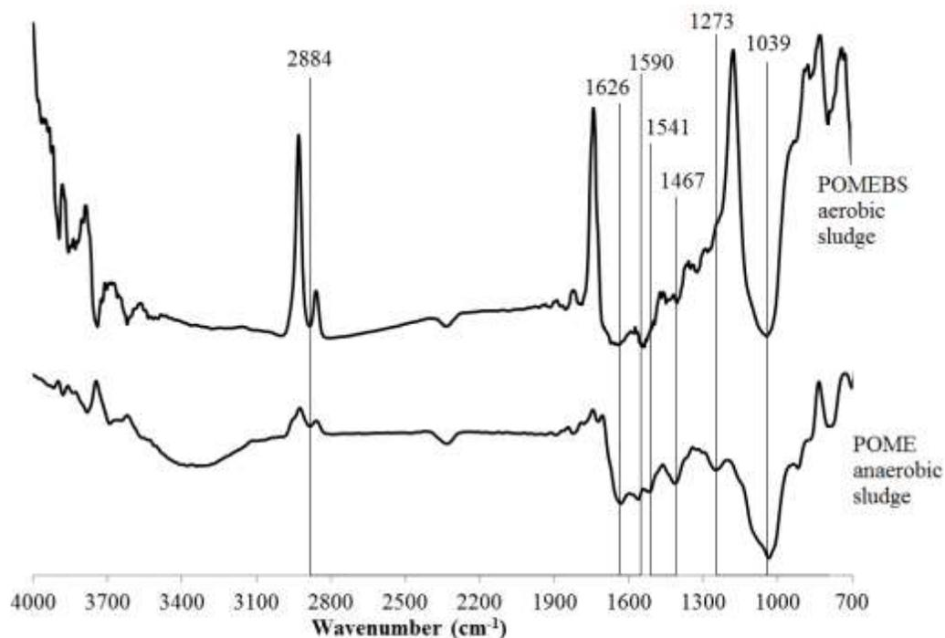
**Fig. 4.** FTIR analysis of POME anaerobic sludge and POMEBS aerobic sludge
