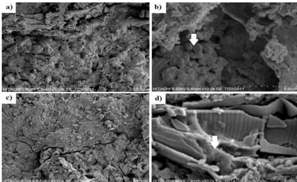
**Fig. 2.** SEM of (a) POME anaerobic sludge at 1000× magnification, (b) POME anaerobic sludge at 10000× magnification, (c) POMEBS aerobic sludge at 1000× magnification, and (d) POMEBS aerobic sludge at 10000× magnification
