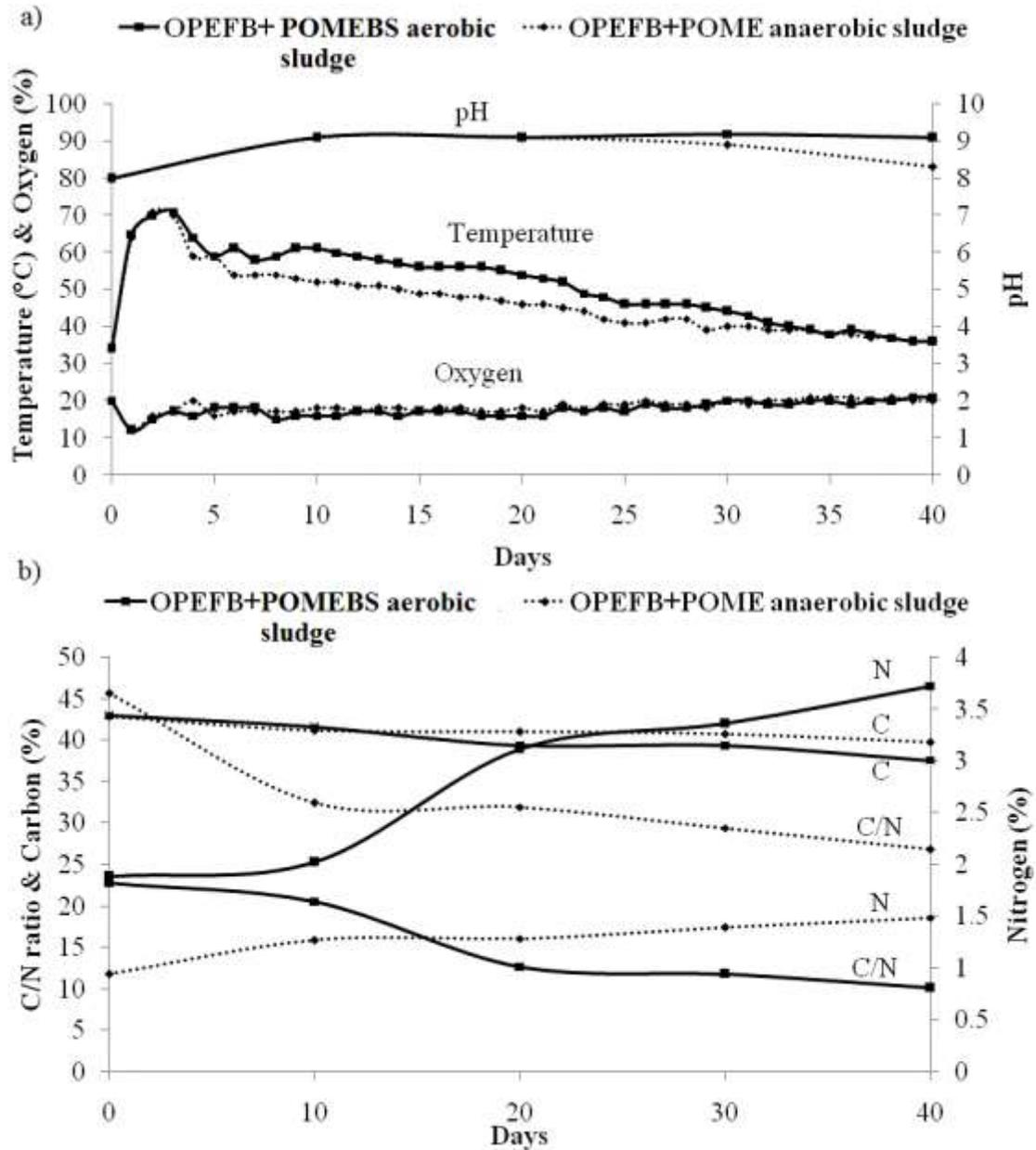
**Fig. 5.** Profile comparison between composting OPEFB with POMEBS aerobic sludge and OPEFB with POME anaerobic sludge for a) temperature, oxygen, and pH; b) carbon, nitrogen, and C/N ratio
