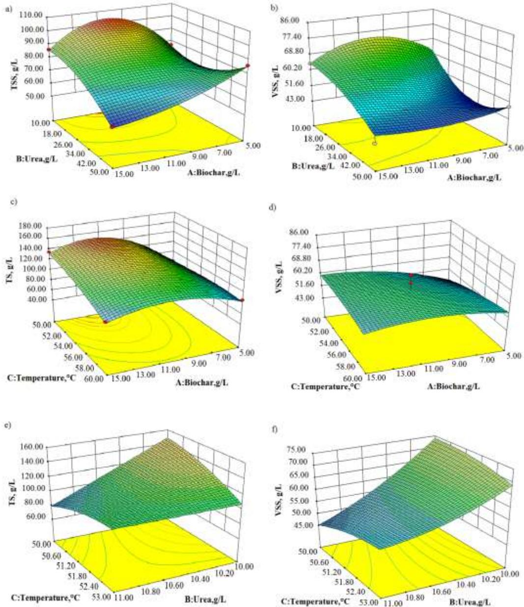
**Fig. 1.** Response surface 3-D plot indicating the effect of interaction between urea and bio-char on a) TS and b) VSS; temperature and bio-char on c) TS and d) VSS; and temperature and urea on e) TS and f) VSS
