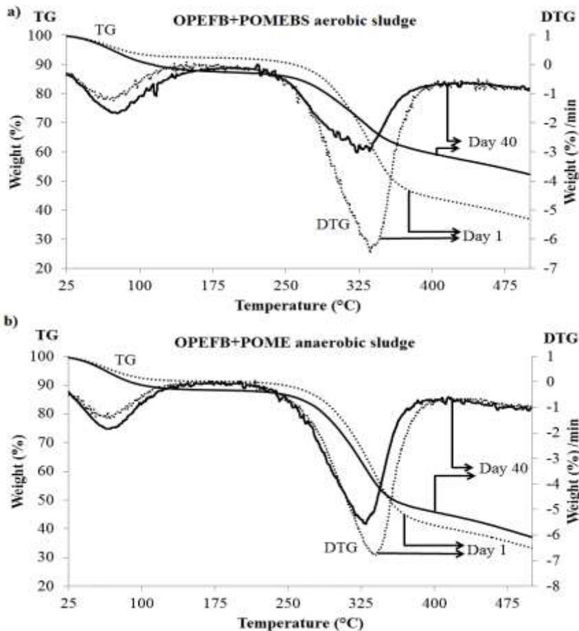
**Fig. 6.** TG and DTG data comparison of composting a) OPEFB with POMEBS aerobic sludge and b) OPEFB with POME anaerobic sludge
